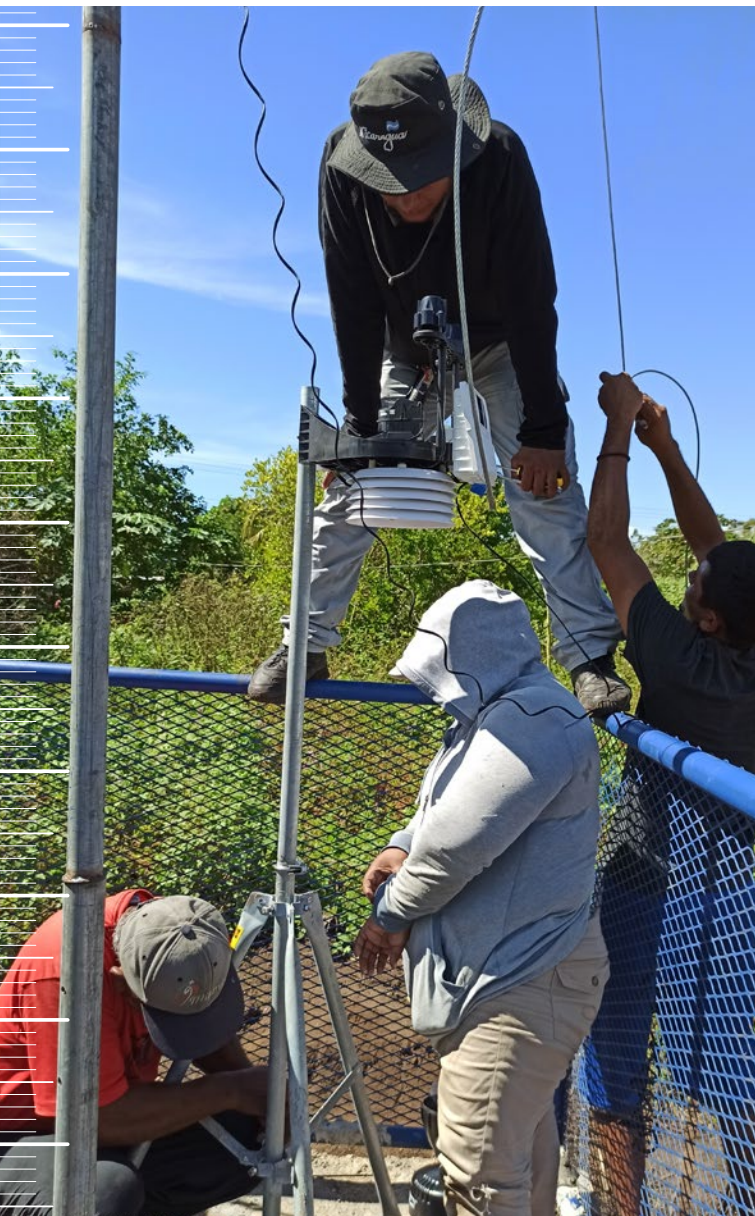
The technical team from INETER installing the new communal weather station in Mechapa, Chinandega, Nicaragua, November 2020 © Felix Rugama, Plan International
