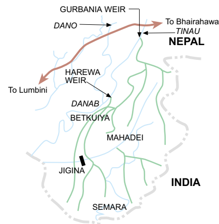
Figure 4b: Layout of traditional Gurbania canal network.
