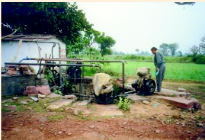
Five pumps on a single well: Tamil Nadu
